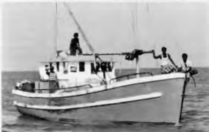
Figure 5. The three principal introduced fishing craft in Sri Lanka: 17.5-ft. outboard-powered skiffs (a), 28-32-ft. boats, the so-called 3.5-tonners (b), and "trawlers" of the Northwest and Abu Dhabi fleets (c). [S. Leatherwood at Chilaw (a) and off Matara (b) and P.A. Folkens off Trincomalee (c)].
