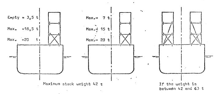
Twistlocks and rods fastened to the second layer
