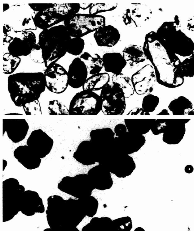
Figure 2. a: 50 % monazite, mounted 1.772, petro x 100, before heat treatment; b: Same, after heat treatment
