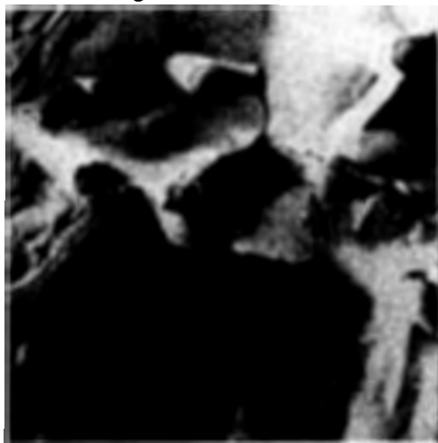
Figure 7. Electron micrograph of UO_2 sintered in a nitrogen atmosphere
