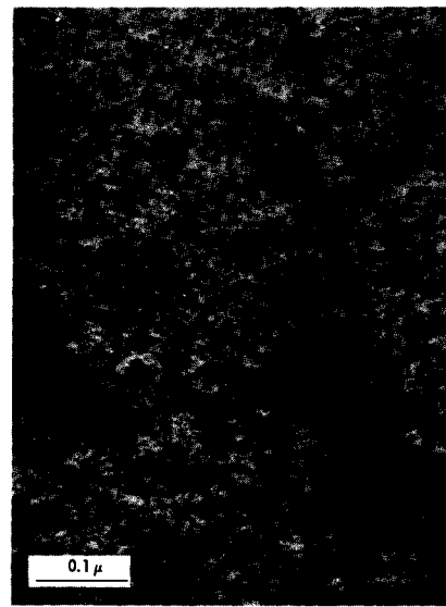
Figure 9. Bright field image of a stoichiometric UO_2 single crystal irradiated at 300^\circ C up to an integrated flux of 10^{17} n/cm^2 (thermal). Numerous clusters of point defects are revealed
