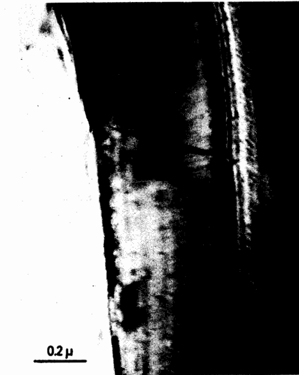
Figure 4. Bright field image of a large needle shaped \text{U}_4\text{O}_9 precipitate in \text{UO}_2 obtained after thermal treatment ( \text{O/U} = 2.007 ). Note the lamellar structure in the needle.
