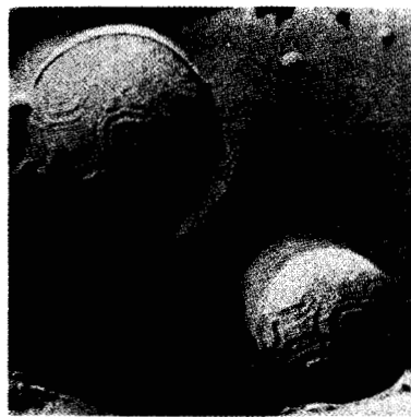
Figure 5. Polyhedra formation in pores in UO_2 which was sintered in an atmosphere of CO_2
