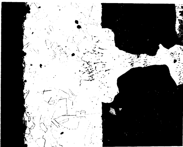
Figure 9. Molten and resolidified steel between the interface of two pellets (etched with aqua regia-glycerol) ( \times 75 )
