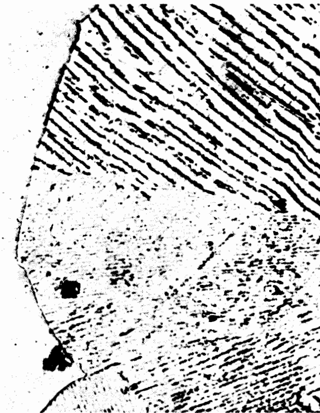
Figure 9. Lamellae with two different directions in one crystal and dihedral angle ( \times 730 )
