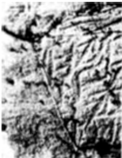
Figure 9. U-2 wt% Nb alloy water quenched from 850 °C. Citric acid electroetching, oblique illumination ( \times 1\ 000 )
