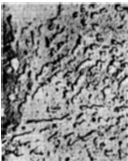
Figure 9 U-2.1 wt% Mo alloy step-annealed at 550 °C and irradiated at 550 °C to a burn-up of 0.40% ( \times 3\,150 )
