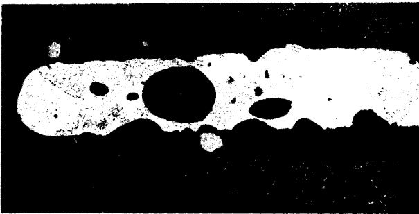
Figure 8. Molten and resolidified steel between the interfaces of two pellets (etched with aqua regia-glycerol) ( \times 75 )
