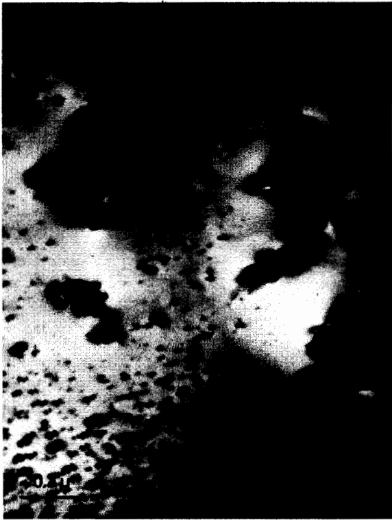
Figure 3. Bright field electron transmission microscopic image of a thin plate of \text{UO}_2 ( \text{O/U} = 2.007 ) showing small coherent precipitates of \text{U}_4\text{O}_9 with a few much larger precipitates of \text{U}_4\text{O}_9 .
