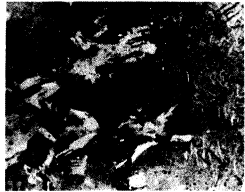
Figure 2. U-0.5 wt% Mo alloy annealed for 10 min at 800 °C and quenched into salt water. Polarised light ( \times 120 )
