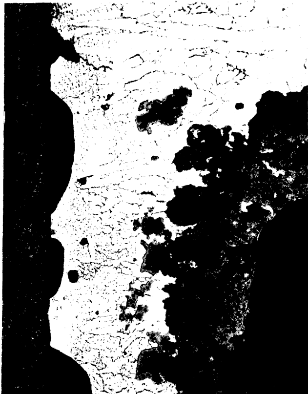
Figure 11. Molten and solidified steel with strong oxidation products (etched with aqua regia-glycerol) ( \times 95 )
