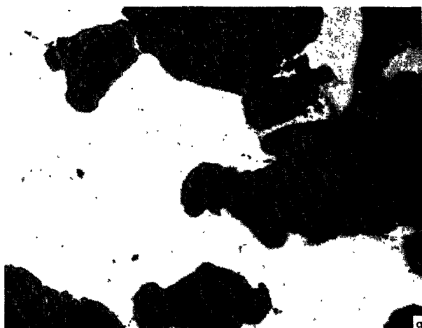
Figure 2a. (U,Pu)O_2 particles in an irradiated cermet which had been fabricated at an early stage of the development programme Burn-up 6 % heavy atoms ( \times 370 )
