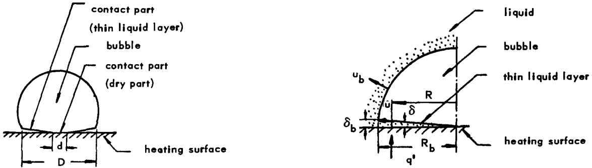
Figure 7. Contact part of bubble on the heating surface
