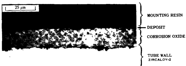
Figure 4. Cross section of film on a fuel sheath typical of recent in-reactor experience Surface temperature 480 \text{ } ^\circ\text{C}
