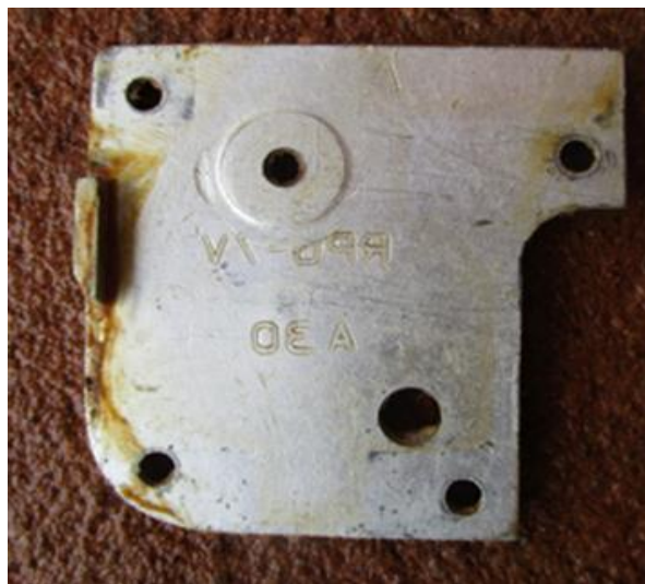
Rear view of the aluminium plate covering the percussion mechanism. The « A 30 » factory marking known to be used by the Sudanese military industry is visible.
