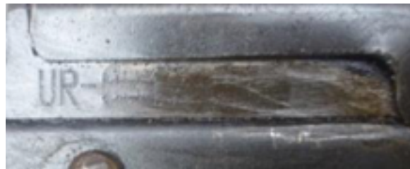
AIM with partially erased serial number.
