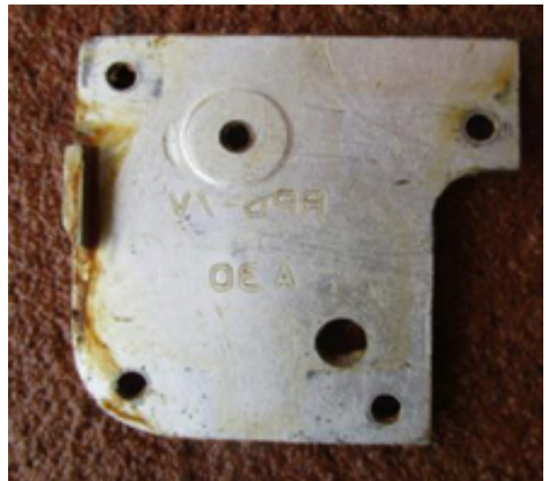
Rear view of the aluminium plate covering the percussion mechanism. The « A 30 » factory marking known to be used by the Sudanese military industry is visible.
