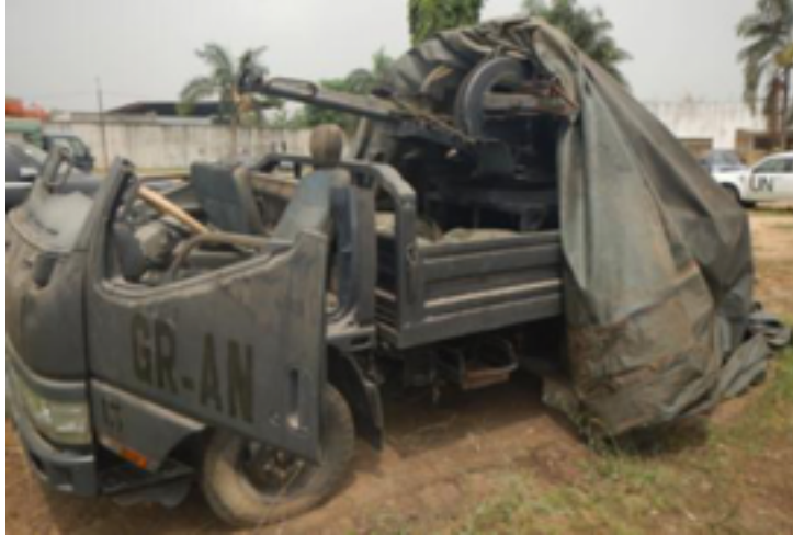
Light truck with ZU-23, twin barrelled anti aircraft autocannon (calibre 23mm)
