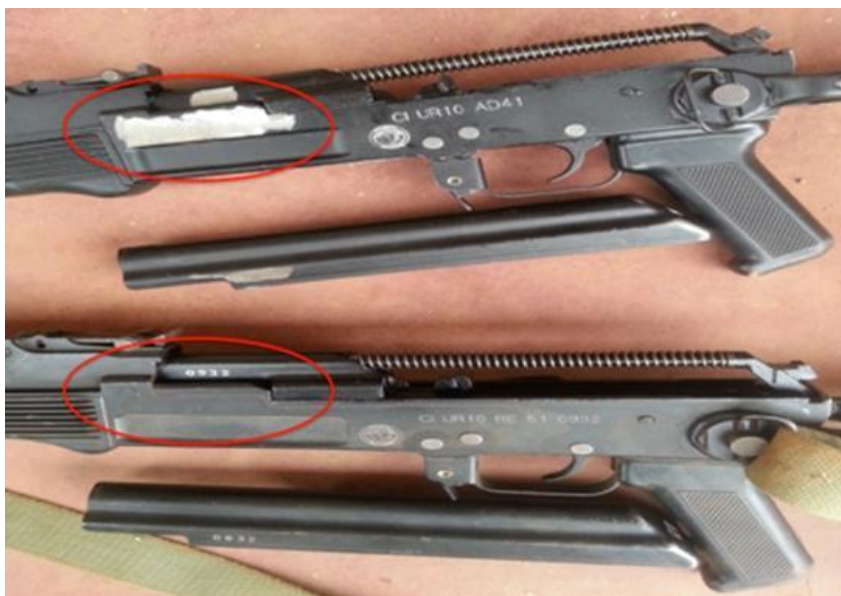
Upper sample: serial numbers mechanically removed. Lower sample: serial numbers still present.
