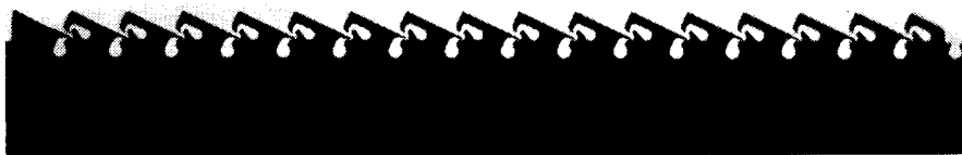
FIG. 4. Metal foil with separation nozzle structures applied by means of photo-etching.
