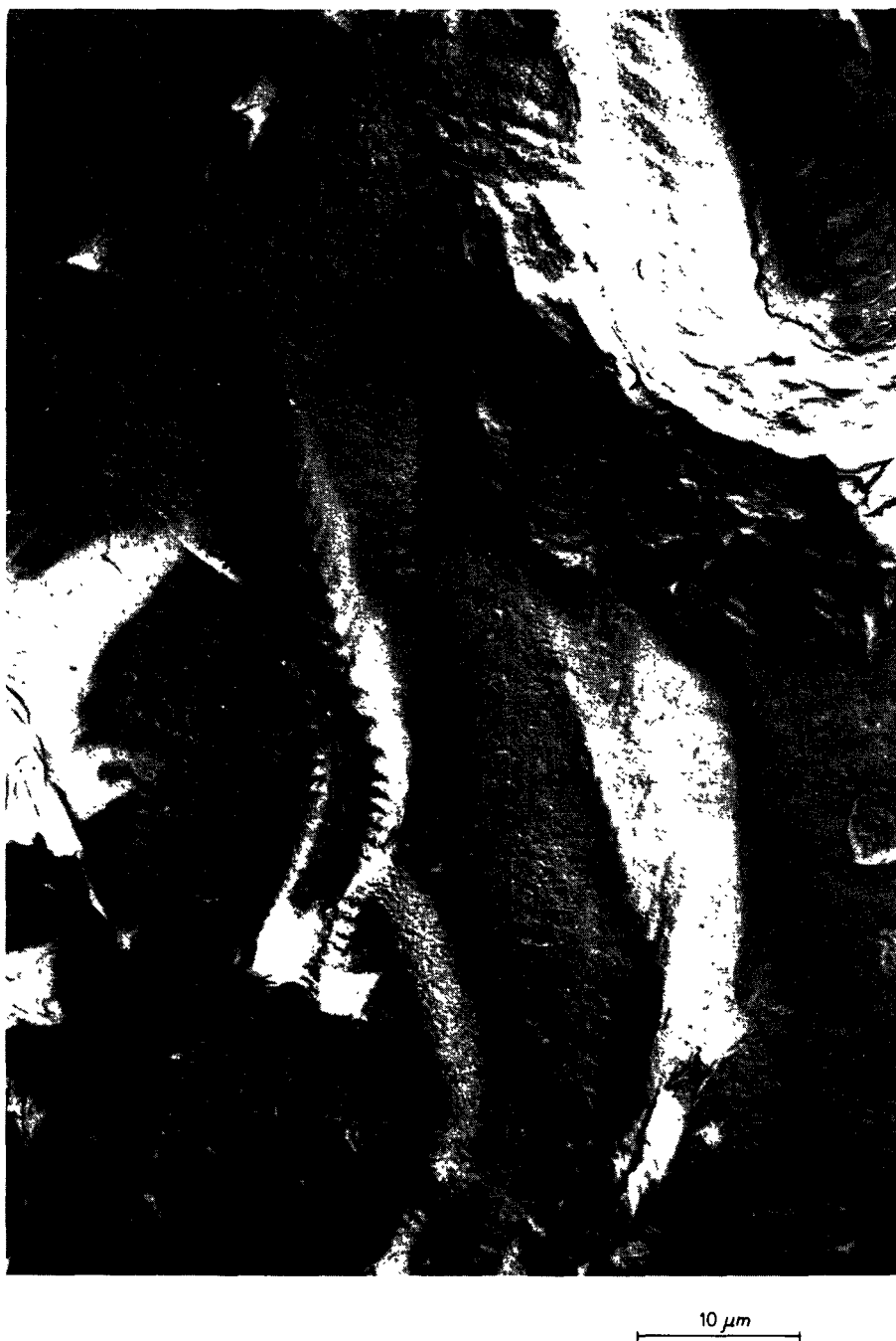
FIG. 4. Microfractograph of fracture surface of fatigued specimen. No. of cycles to fracture: 3960.
