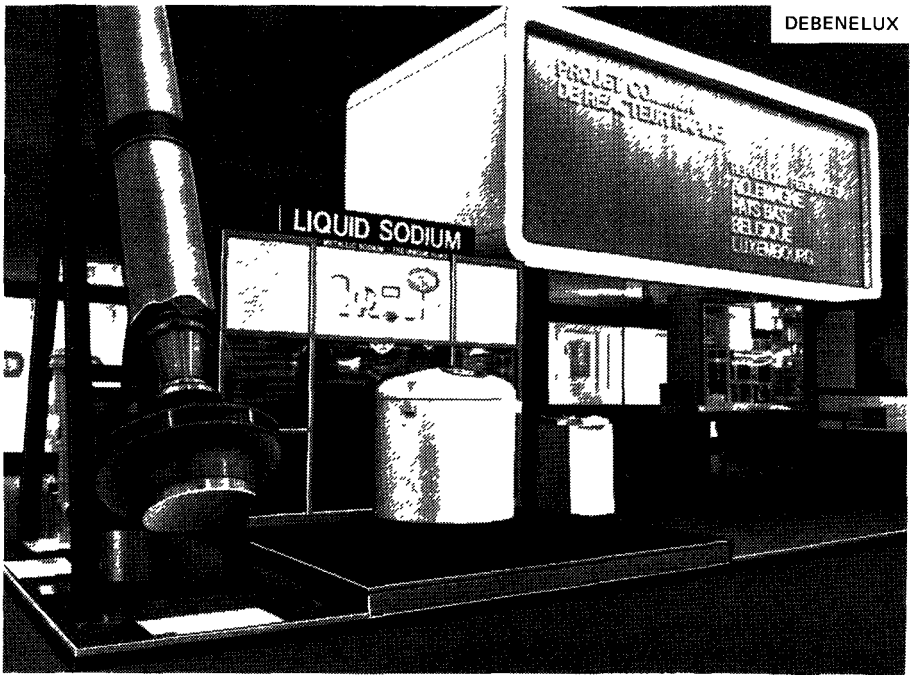
View of Debenelux Stand showing, left to right, the impeller of the 5000 m 3 /h sodium pump, the liquid sodium demonstration and the model of the 300 MW(e) SNR prototype.
