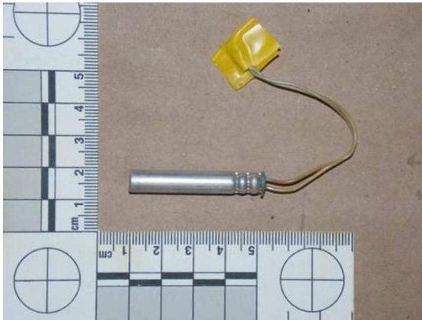
C-DET cap recovered from the 5 September 2013 incident at Hawlwadaag (below)
