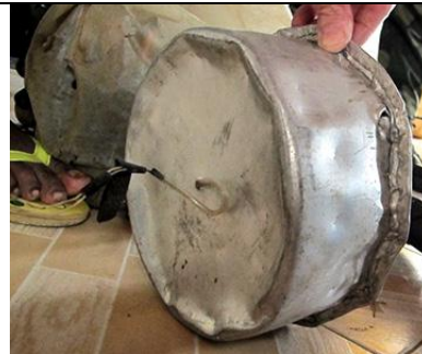
View of the bottom of the IED, showing the command wire entering the pot.
