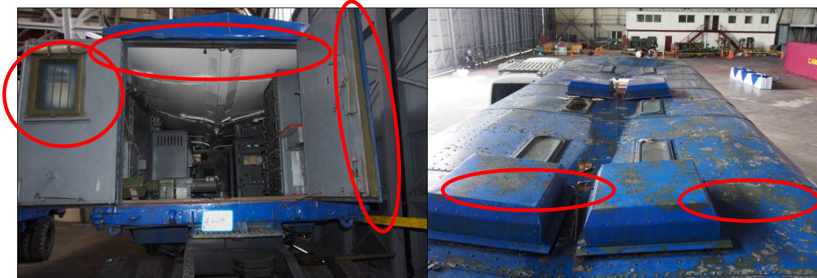
Figure 2: Original paint scheme inside (left) and revealed by damage (right)
