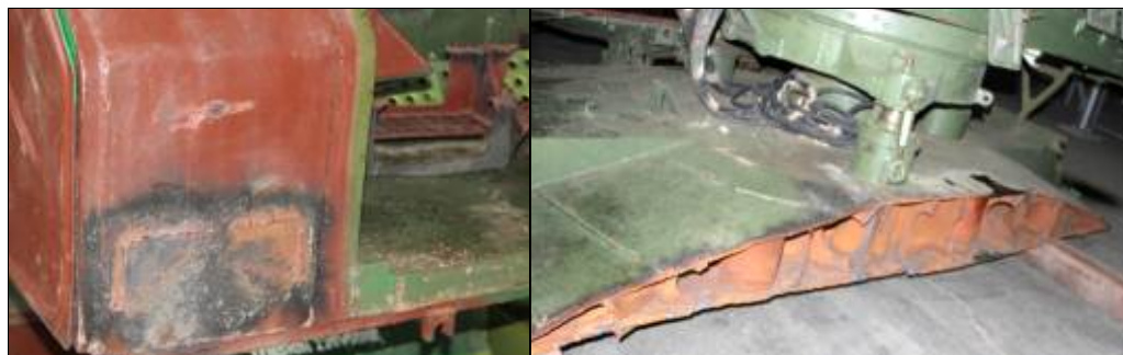
Figure 17: SA-2 and SA-3 parts chopped off in order for launchers to fit into the containers
