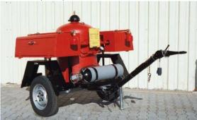
5. Fire extinguishers composed of a non-rollable pressure drum and equipment, transported unpacked and handled e.g. by fork lift or crane when loaded or unloaded.
