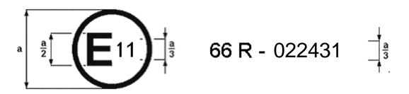
The above approval mark affixed to a vehicle shows that the vehicle type concerned has, with regard to the strength of the superstructure, been approved in the United Kingdom (E11) pursuant to Regulation No. 66 under approval number 022431. The first two digits of the approval number indicate that the approval was granted in accordance with the requirements of the 02 series of amendments to Regulation No. 66."
