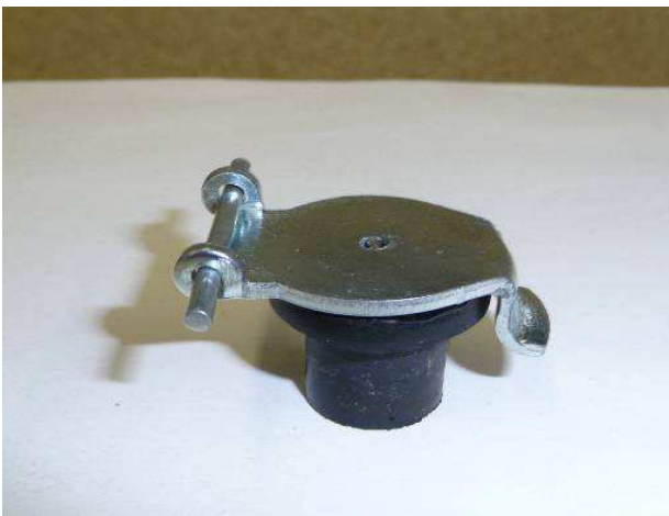
Fig 4: Rubber plug and metal clack to seal the receptacle
