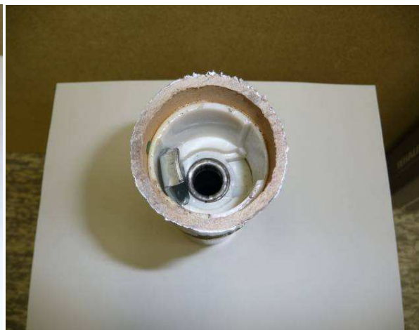
Fig. 5: Lock mechanism for opening by turning a plastic ring
