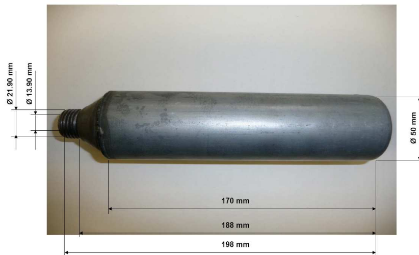
Fig. 3: Pressurized receptacle made of steel, contained in 80 cm shooters
