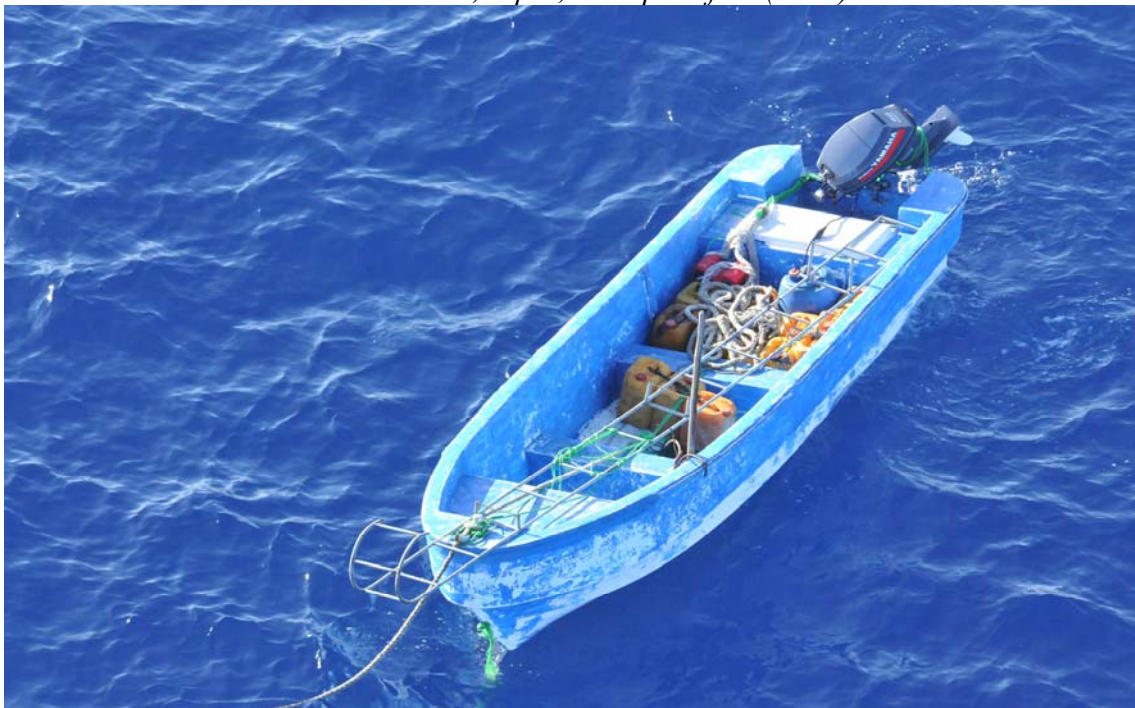
Typical pirate attack skiffs with 60HP Yamaha outboard engine, ladder with welded bow, grappling hook, ropes, and spare fuel (2010)
