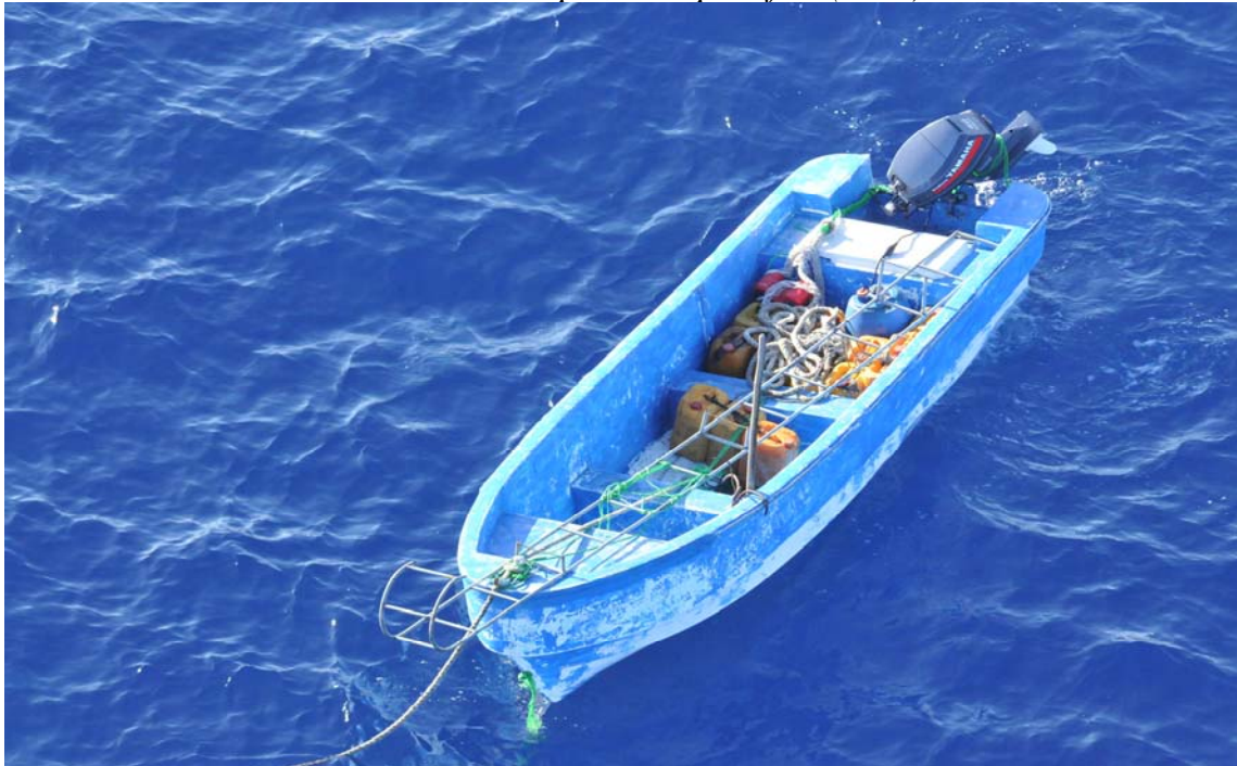
Typical pirate attack skiffs with 60HP Yamaha outboard engine, ladder with welded bow, grappling hook, ropes, and spare fuel (2010)
