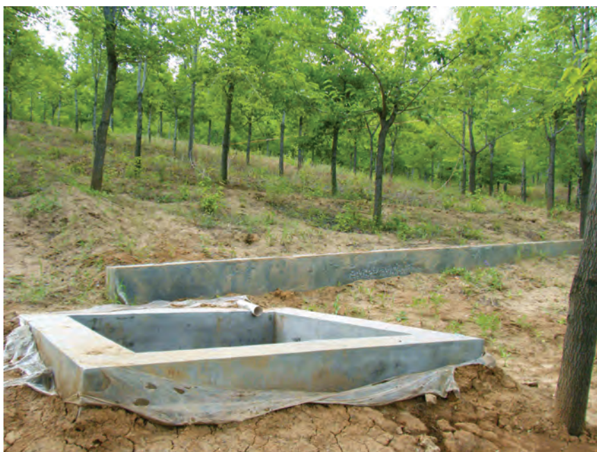
Plate 5.2.1 Soil erosion observation plot installed at the Eucommia plantation
