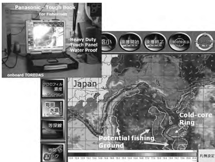
Figure 3.4.6 Onboard PC system and display of an SST image from the onboard GIS.
