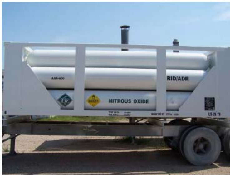
Figure 4: 20-foot-long MEGC (half-length and full-height – 10 tubes)
