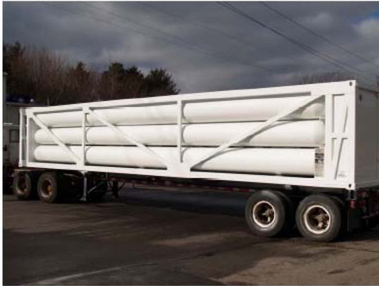
Figure 1: 40-foot-long MEGC (full-length and full-height – 12 tubes)
