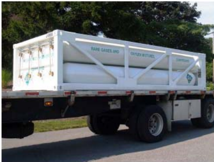
Figure 6: 20-foot-long MEGC (half-length and half-height – 8 tubes)
