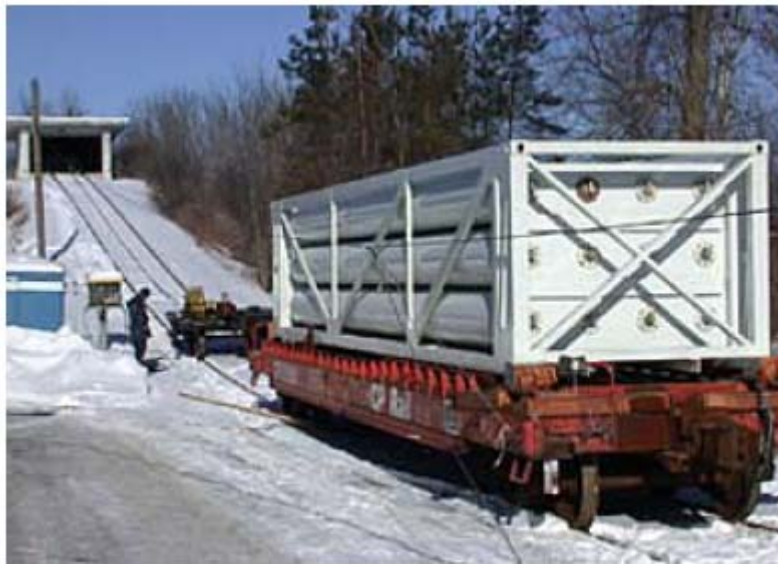
Figure 2: MEGC undergoing an impact test
