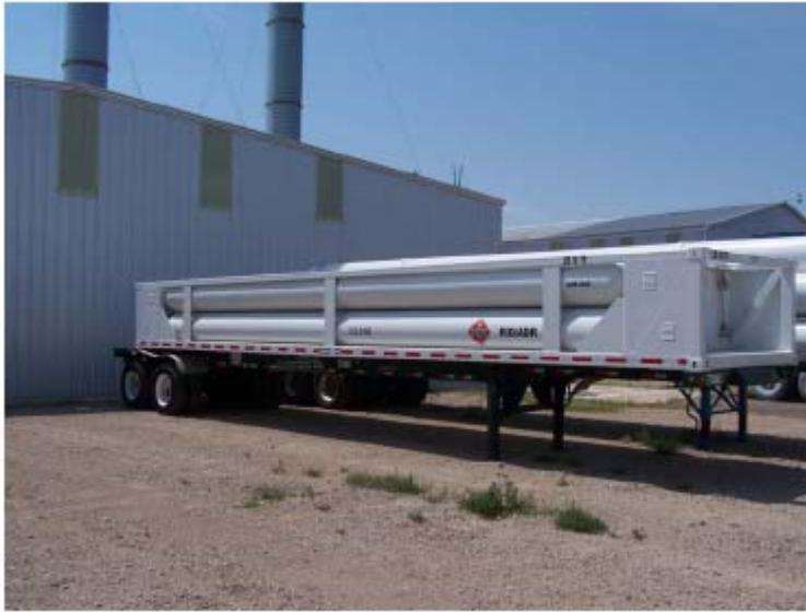
Figure 3: 40-foot-long MEGC (full-length and half-height – 8 tubes)
