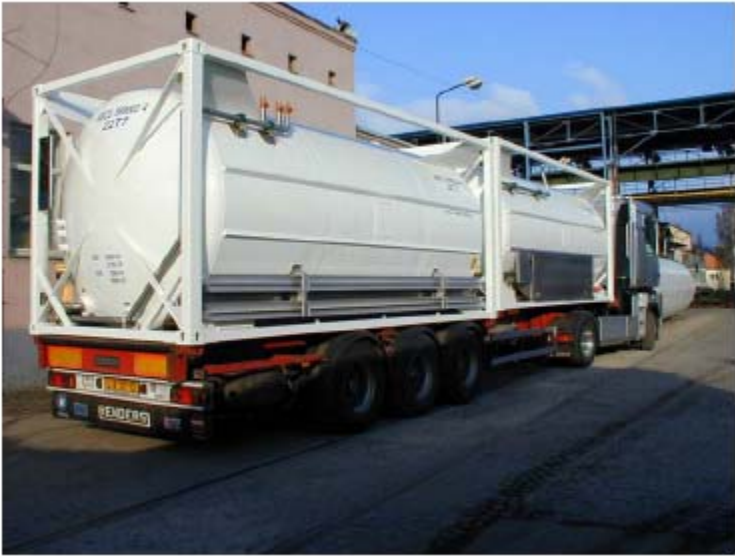
Figure 10: Vacuum-jacketed cryogenic portable tank
