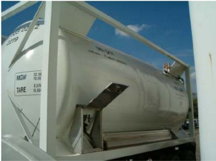
Figure 11: Vacuum-jacketed cryogenic portable tank
