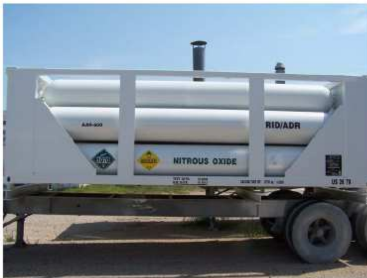
Figure 4: 20-foot-long MEGC (half-length and full-height – 10 tubes)
