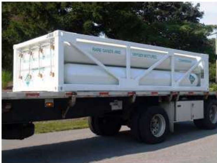
Figure 6: 20-foot-long MEGC (half-length and half-height – 8 tubes)
