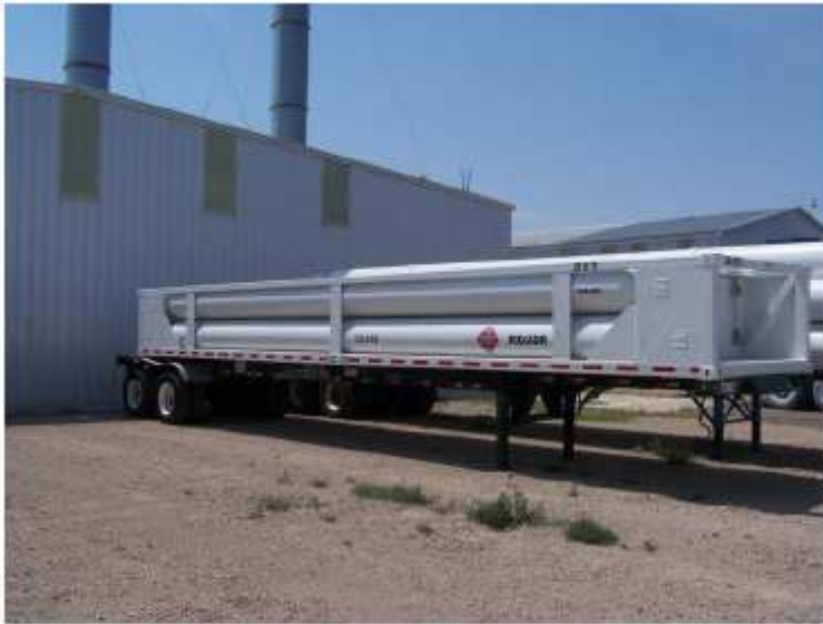
Figure 3: 40-foot-long MEGC (full-length and half-height – 8 tubes)
