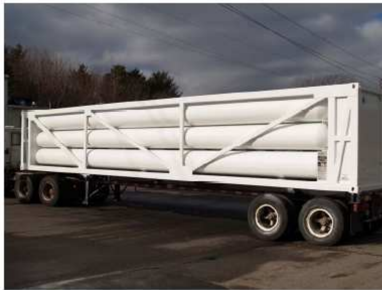
Figure 1: 40-foot-long MEGC (full-length and full-height – 12 tubes)
