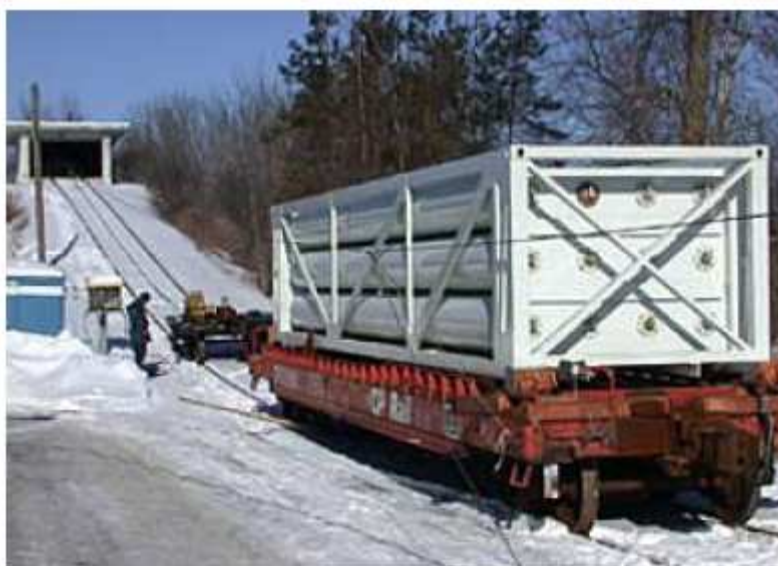
Figure 2: MEGC undergoing an impact test
