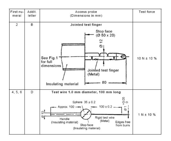
Table 1 - Access probes for the tests for protection of persons against access to hazardous parts
