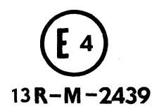
The above approval mark affixed to a vehicle of categories M<sub>2</sub> and M<sub>3</sub> shows that, pursuant to Regulation No.13, the vehicle type concerned has with regard to braking, been approved in the Netherlands (E.4) under approval number 2439 and that it has undergone the type-II bis test.
