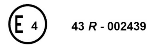
Approval number for uniformly toughened glass in accordance with the current provisions of UNECE Regulation No. 43.
