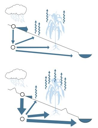
Figure 2.1: Landscape water balance flows a) without rainwater harvesting, and b) an example of flow paths with rain water harvesting interventions with water partitioning points at the soil surface (1), and in the soil (2). Rainwater harvesting is principally about managing water partitioning in these points.
