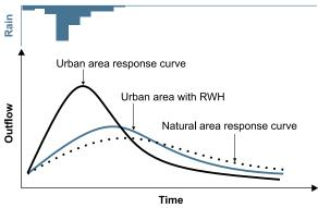
Figure 2.2: principal flow response curve from an urban catchment with and without rainwater harvesting in place, showing the effect of slower flow through the landscape (contributed by K. König)
