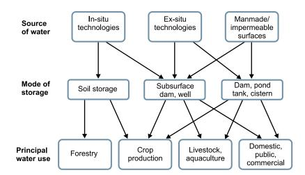
Figure 2.5: Schematic of rainwater harvesting technologies based on source of water and water storage type Modified after SIWI, 2001
