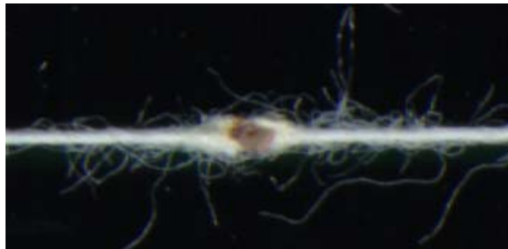
Figure 2.17: A seedcoat nep in yarn
