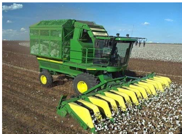
Figure 2.2: Typical stripper harvester for cotton
