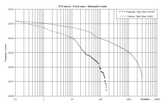
**Figure 4:** Example of an FN graph for the societal risk of the main substances ammonia and chlorine for a road tunnel (from[11])
