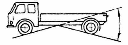
4.7.5.4. "<u>Ground clearance between the axles</u>" means the shortest distance between the ground plane and the lowest fixed point of the vehicle.
