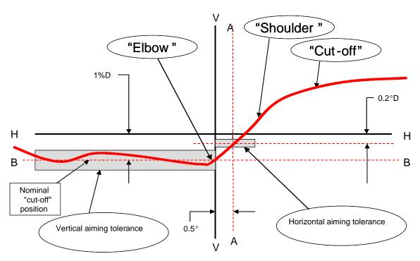
Note: The scales are different for vertical and horizontal lines.
