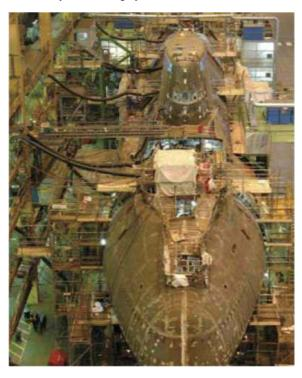
HMS ASTUTe under construction at BAe Systems Submarines, Barrow-in-Furness (picture courtesy of BAe Systems)
