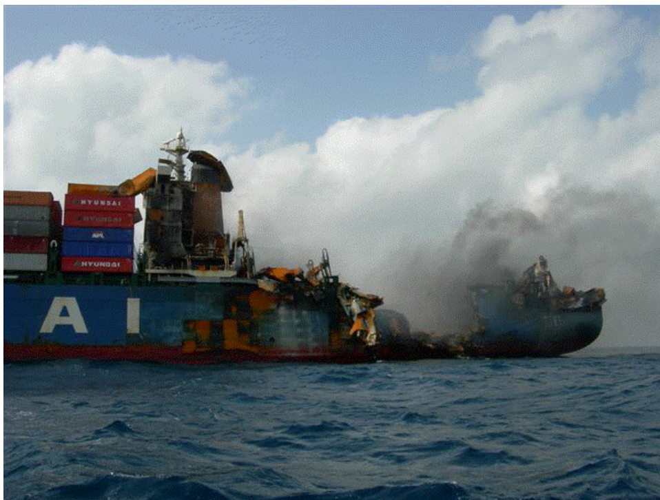
Image 2: MV Hyundai Fortune damage aft
