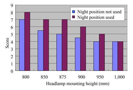
Figure 4 Glare from the following vehicle (the distance between vehicles: 5 m)
