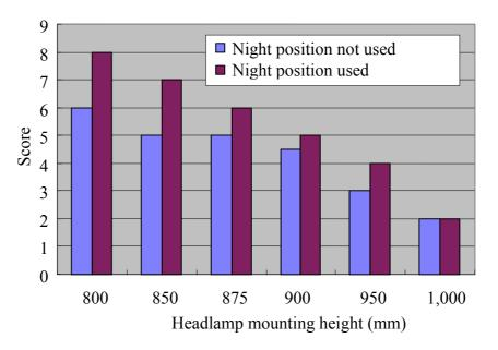
Figure 3 Glare from the following vehicle (the distance between vehicles: 3 m)
