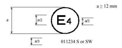
The above approval mark shows that the tyre concerned has been approved in the Netherlands (E4) pursuant to Regulation No. 117 (marked by S (rolling sound) or both S (rolling sound) and W (wet adhesion), under approval number 011234. This indicates that the approval is for S or both SW. The first two digits of the approval number (01) indicate that the approval was granted according to the 01 series of amendments.
