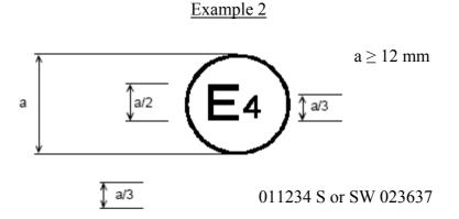
The above approval mark shows that the tyre concerned has been approved in the Netherlands (E4) pursuant to Regulation No. 117 (marked by S (rolling sound) or SW (rolling sound and wet adhesion)), under approval number 011234 and Regulation No. 30 under approval number 023637. The first two digits of the approval number (01) indicate that the approval was granted according to the 01 series of amendments, but Regulation No. 30 included the 02 series of amendments.
