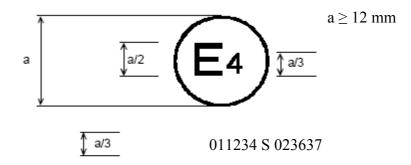
The above approval mark shows that the tyre concerned has been approved in the Netherlands (E4) pursuant to Regulation No. 117 (marked by S (rolling sound)), under approval number 011234 and Regulation No. 30, under approval number 023637. The first two digits of the approval number (01) indicate that the approval was granted according to the 01 series of amendments, but Regulation No. 30 included the 02 series of amendments.
