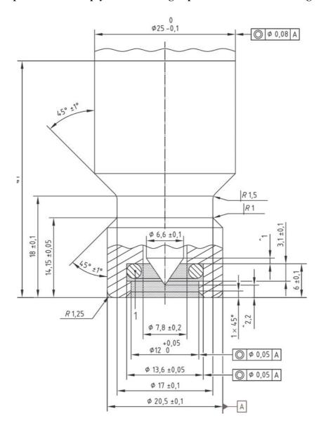
Fig. 1 Standard connector (receptacle) dimensions [mm]"
