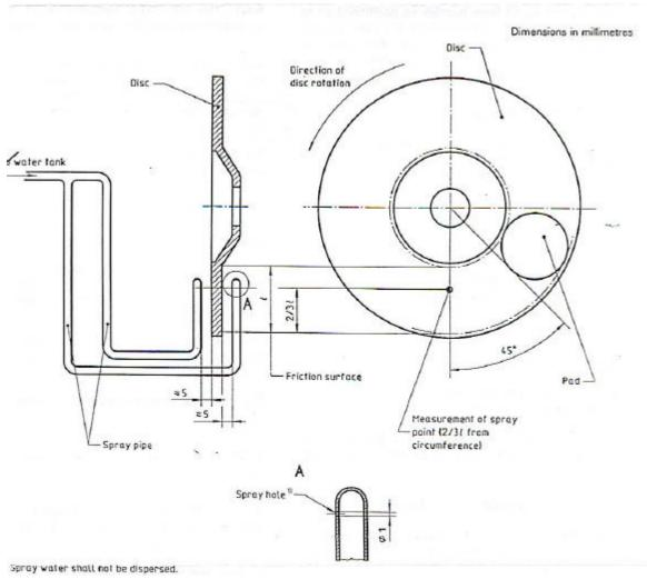
(a) Disc brakes: Sketch of water spray equipment.
