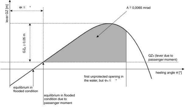
(iii) non-watertight openings shall not be immersed before the equilibrium position has been reached; if such openings are immersed before this point, the rooms affording access are deemed to be flooded for damaged stability calculation purposes.
