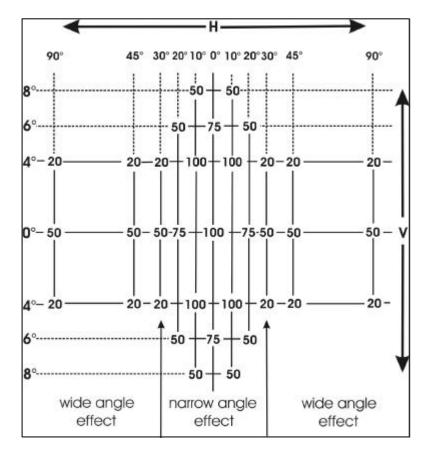
Minimum horizontal angular range of category "narrow angle effect" is  $30^{\circ}$  left to  $30^{\circ}$  right and for category "wide angle effect"  $90^{\circ}$  directed outwards the vehicle and  $30^{\circ}$  to the inside.
