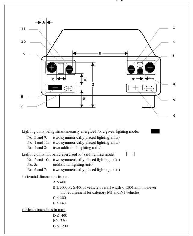
Apparent surfaces of lighting units 1 through 11 of an AFS (example)
