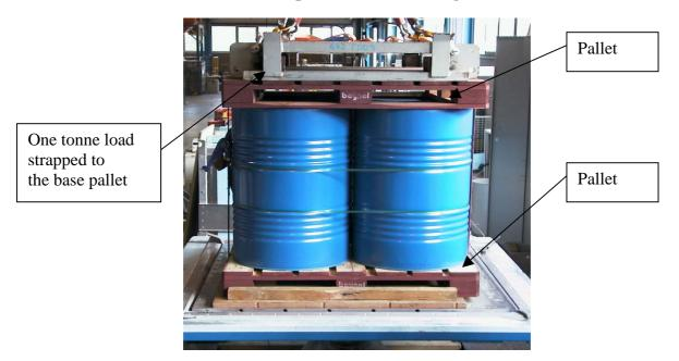
Pallet secured on the vibrating table
