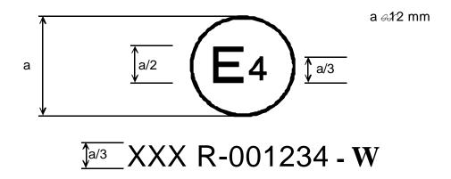
The above approval mark, affixed to a pneumatic tyre shows that the tyre concerned has been approved in the Netherlands (E4) pursuant to Regulation No. XXX (-W) under approval number 001234. The first two digits of the approval number (00) indicate that the approval was granted according to the requirements of this Regulation in its original form.
