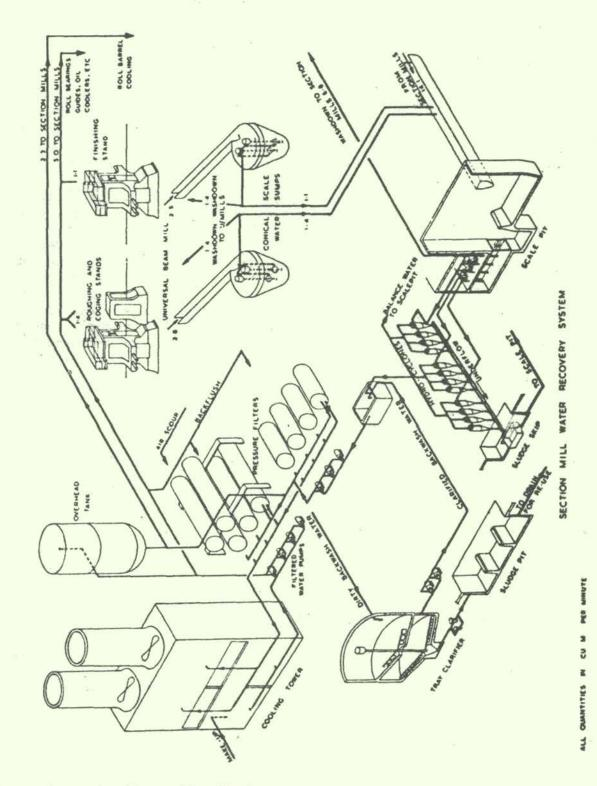
DIAGRAM OF SECTION MILL WATER RECOVERY SYSTEM
