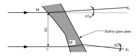
Figure 6: Diagrammatic representation of optical distortion
