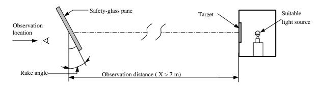
Figure 12: Arrangement of apparatus
