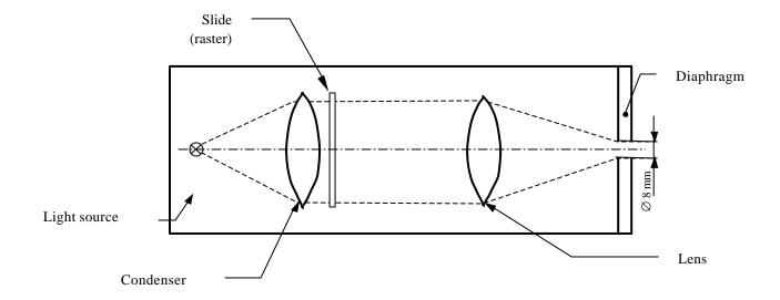
Figure 7: Optical arrangement of the projector
