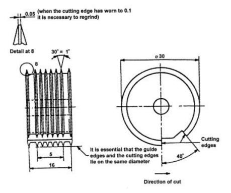
Figure 24: Tool with six blades
