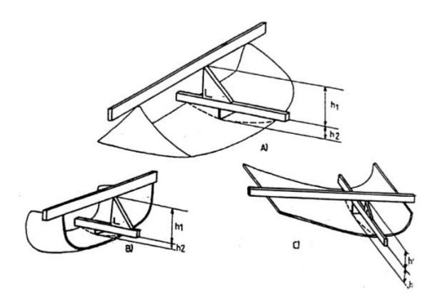
Figure 1: Determination of the height of segment 'h'
