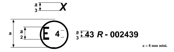
The above approval mark affixed to a rigid plastic double glazed unit shows that the component concerned has been approved in the Netherlands (E 4) pursuant to Regulation No. 43 under approval No. 002439. The approval number indicates that the approval was granted in accordance with the requirements of Regulation No. 43.
