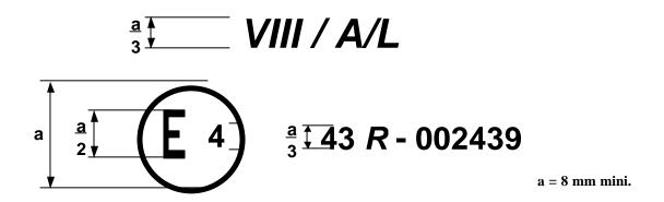
The above approval mark affixed to a rigid plastic glazing pane for forward facing panels with a light scatter not exceeding 2 per cent after 1000 cycles on the outer surface and 4 per cent after 100 cycles on the inner surface shows that the component concerned has been approved in the Netherlands (E 4) pursuant to Regulation No. 43 under approval No. 002439. The approval number indicates that the approval was granted in accordance with the requirements of Regulation No. 43.
