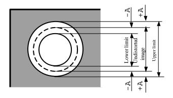
Figure 10: Design for a suitable checking template
