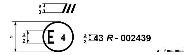
The above approval mark affixed to a treated laminated-glass windscreen shows that the component concerned has been approved in the Netherlands(E 4) pursuant to Regulation No. 43 under approval No. 002439. The approval number indicates that the approval was granted in accordance with the requirements of Regulation No. 43.
