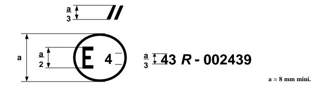
The above approval mark affixed to an ordinary laminated-glass windscreen shows that the component concerned has been approved in the Netherlands (E 4) pursuant to Regulation No. 43 under approval No. 002439. The approval number indicates that the approval was granted in accordance with the requirements of Regulation No. 43.
