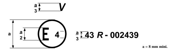
The above approval mark affixed to a glass pane other than a windscreen to which the requirements of annex 3, paragraph 9.1.4.2., are applicable shows that the component concerned has been approved in the Netherlands (E 4) pursuant to Regulation No. 43 under approval No. 002439. The approval number indicates that the approval was granted in accordance with the requirements of Regulation No. 43.
