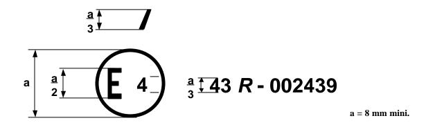
The above approval mark affixed to a toughened-glass windscreen shows that the component concerned has been approved in the Netherlands (E 4) pursuant to Regulation No. 43 under approval number 002439. The approval number indicates that the approval was granted in accordance with the requirements of Regulation No. 43.
