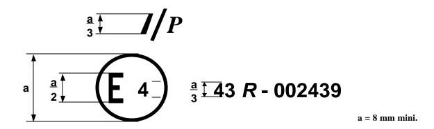
The above approval mark affixed to a toughened-glass windscreen faced with plastics material shows that the component concerned has been approved in the Netherlands (E 4) pursuant to Regulation No. 43 under approval No. 002439. The approval number indicates that the approval was granted in accordance with the requirements of Regulation No. 43.
