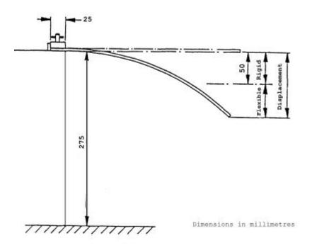
Figure 23: Arrangement of flexibility test
