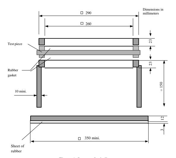
Figure 1: Support for ball tests
