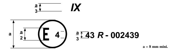
The above approval mark affixed to a flexible plastic glazing pane shows that the component concerned has been approved in the Netherlands (E 4) pursuant to Regulation No. 43 under approval No. 002439. The approval number indicates that the approval was granted in accordance with the requirements of Regulation No. 43.
