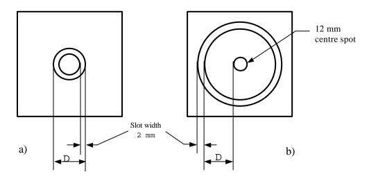
Figure 11: Dimensions of targets
