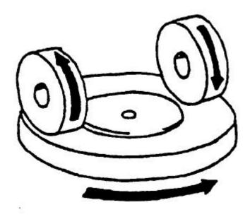
Figure 4: Diagram of abrading instrument
