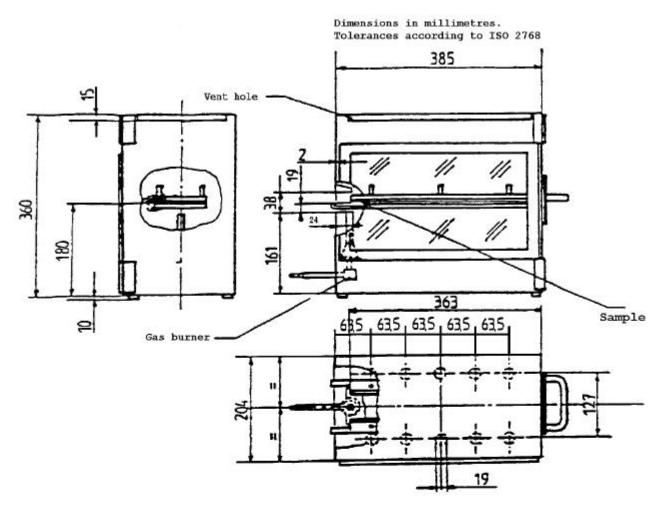
Figure 16: Example of combustion chamber
