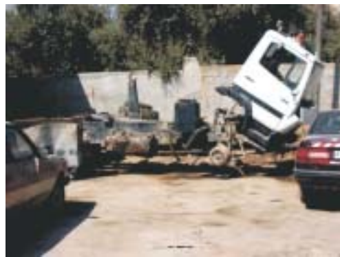
Solid waste truck in state of disrepair
