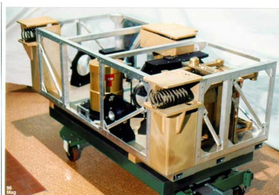
FIG. 2: The SAFIRE Fourier Transform Spectrometer
