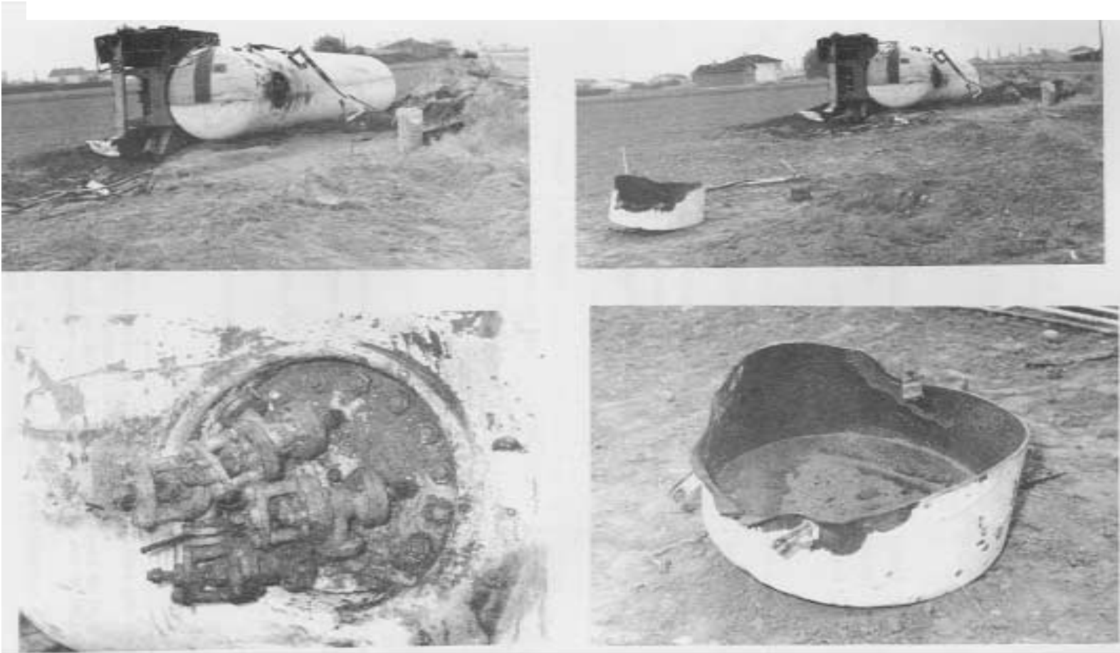
APPENDIX 8 – Chlorine Tanker Roll Over – The vulnerability of everything external to the shell can be clearly seen.
