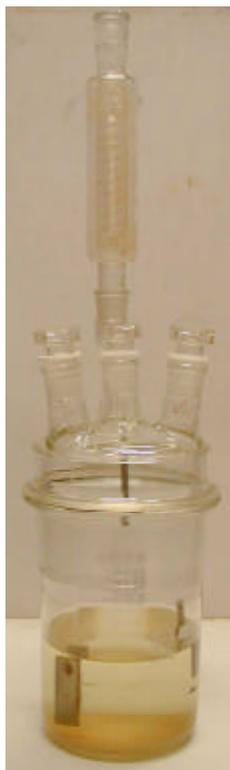
Figure 37.4.2: Exposure receptacle with reflux condenser
