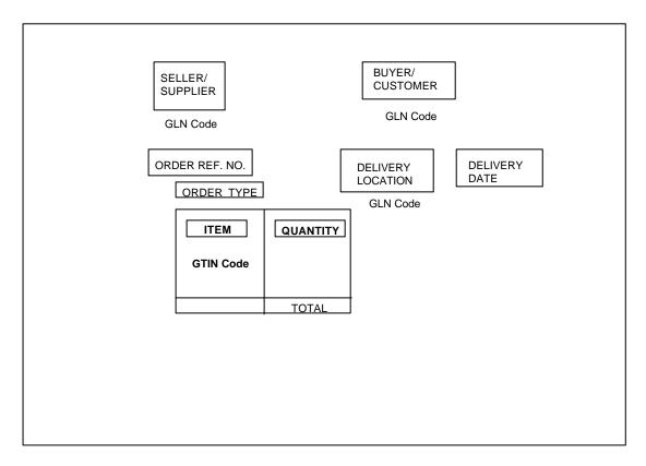
Diagram 3.1: Basic Components of a Simpl-eb Order
